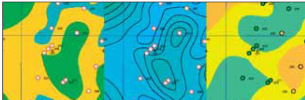
Figure 6 'Hydrocarbon Potential Map' (left), 'Hydrocarbon Contour Map' (centre) and 'Noise & Quality Map' (right). The circles, labelled by identification numbers, indicate measurement locations on a selected area of 2 km x 2 km including multiple measurements (e.g. 225, 226, 227) taken at the position of the lower left circle. The green filled circles in the 'Noise & Quality Map' indicate highest quality measurements.
