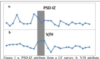
Figure 1 a. PSD-IZ attribute from a LF survey. b. V/H attribute from the same survey. The grey box indicates surface projected HC locations.
