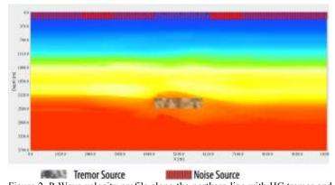
Figure 2. P-Wave velocity profile along the northern line with HC tremor and noise source locations. Red=high velocity, blue=low velocity. At surface darker red indicates stronger noise source.
