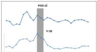
Figure 3 a. synthetic PSD-IZ profile (SNR=0.10). b. Synthetic V/H profile (SNR=0.10). The grey box indicates surface projected HC locations.
